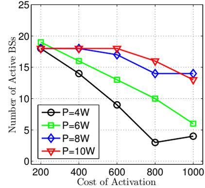
**Figure 5: Number of active BSs versus transmission power and activation cost in a network with uniform user distribution.**
