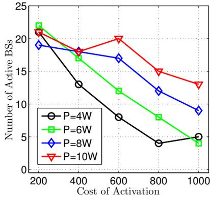
Figure 6: Number of active BSs versus transmission power and activation cost in a network with uniform user distribution.
